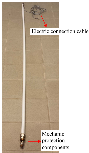
Fig. 5. The experimental prototype of the proposed water-level sensor for measuring a maximum water level of 2 m.
