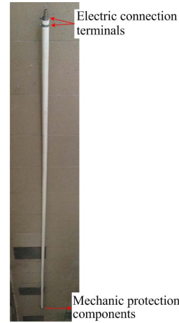
Fig. 7. An experimental prototype of the proposed sensor for a measuring range of 4 m.
