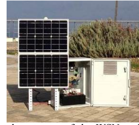
Fig. 6. The experimental prototype of the WSN node power-supply system, which has been designed according to the proposed optimization technique.
